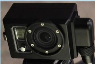
The system includes the very latest and innovative **GoPro 4 HD camera** integrated within a durable metal subsea enclosure rated to 100m depth that ensures optimum imaging performance, small size, reliability and durability in the ocean environment.
