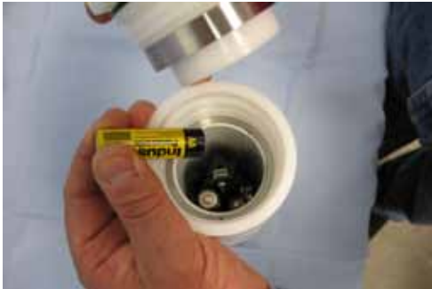
Users can easily replace the commercial batteries in the KILO-DIO.
