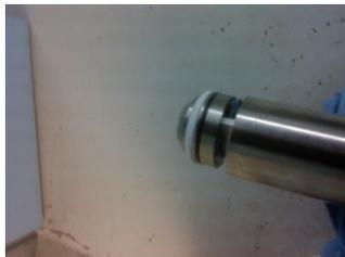
It is recommended that users make use of a vice or another stabilizing device and gently tap on the protruding screw with a rubber mallet until there is enough of the head of the sable exposed to get a firm grip on with your hands and pull the internal chassis out horizontally. Be careful not to scratch the inside of the titanium case where the O-ring seats.
