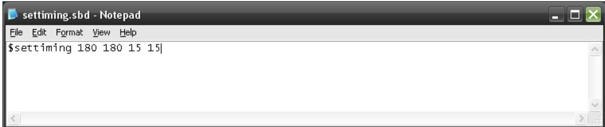
**180 = Normal GPS Check** interval is the number of minutes between Sable's GPS location acquisition after the first hour of power up and before it goes underwater
