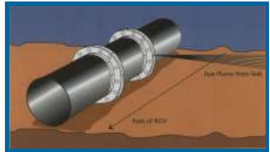
Dye-plume leaking from pipeline flange
