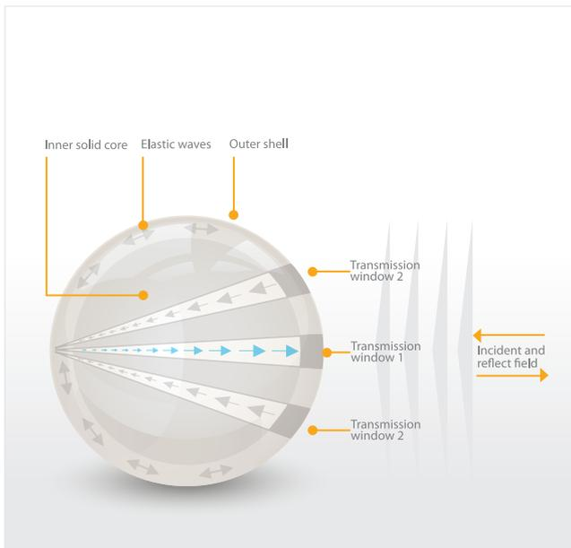
SonarBell™ operates by focusing and reflecting acoustic energy, much as a lens or mirror can focus light. Just like a lens or mirror, SonarBell™ is a completely passive device.
